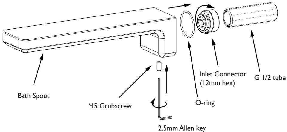
NOTE - Maximum hole diameter through wall for G1/2 tube is 22mm (7/8")
