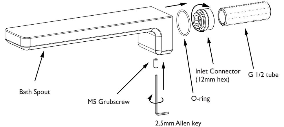
NOTE - Maximum hole diameter through wall for G1/2 tube is 22mm (7/8")
