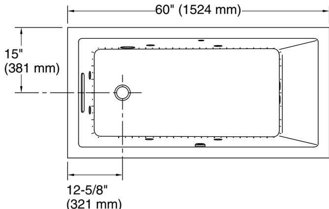
No change in measurements if connected with drain illustrated. (K-7271)
