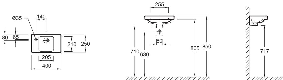
Product Specification: Handwash basin. E4759C-X5. Collection: ODÉON UP. DIMENSIONS: 40 x 25 cm. WEIGHT: 5.5 kg. MATERIAL: Ceramic. INSTALLATION TYPE: Self-supporting. TAP DRILLING: 1 tap hole. INSTALLATION: STANDARD. OVERFLOW: Without overflow hole.
