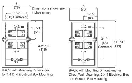
Figure-2 Mounting Dimensions.
