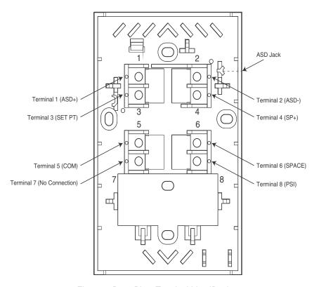
Figure-3 Base Plate Terminal Identification.
