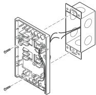
2 X 4 Electrical Box Pigtail Mounting.
