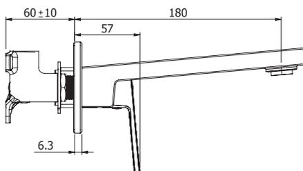
**CONSTRUCTION:** Brass body & spout - metal plate
